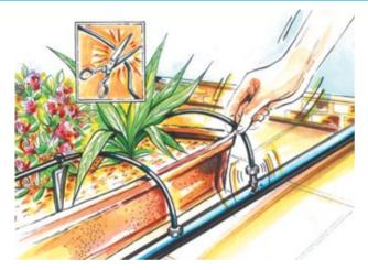
Cut lengths of the 1/4" hose to measure. After making holes in the 1/2" tube for each branching, connect each length to the 1/2" tube by means of the 2-way connector (code 91155). For greater flexibility and control of water flow to each branching, a tap can also be used for each feeding tube.
