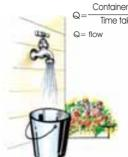
Q=  $\frac{\text{Container capacity (e.g. 10 litres)}}{\text{Time taken (e.g. 20 seconds)}} \times 60 = \frac{10}{20} \times 60 = 30 \text{ litres/min}$
