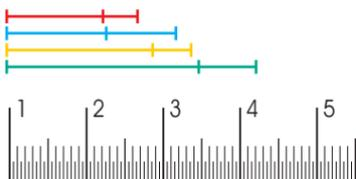
How to immediately find the diameter in inches of a hose. Use this practical conversion table for inside and outside diameters. There is also a graduated scale along the edge of the page: place it against the inside diameter, then compare it with the length of the coloured lines. The red line corresponds to 1/2", the blue to 5/8", the yellow to 3/4" and the green to 1".
